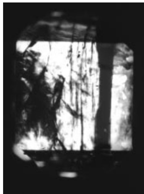
Figure 3. Photograph of KDP crystal (8 (H) × 5 (W) × 3 (D) mm 3 ) at 195 °C viewed between crossed polarizers. Hemispherical, extinguished (black) region at left is II'. Extinguished band in right half of crystal is untransformed II. Bright regions are polycrystalline.
